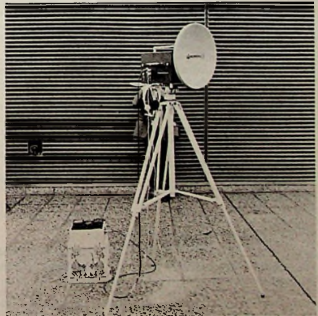
Ontvangparabool en converter in experimentele opstelling.
